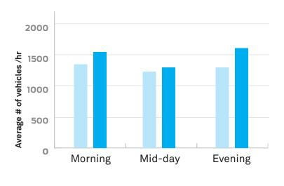
Vehicular travel times did not increase along the corridor despite the allocation of space to the cycle lane. In certain cases the capacity of vehicular volumes on the street increased because of the alignment/reduction of the travel lane widths. This proves that efforts to create dedicated space for cyclists can also effectively improve vehicular movement.
