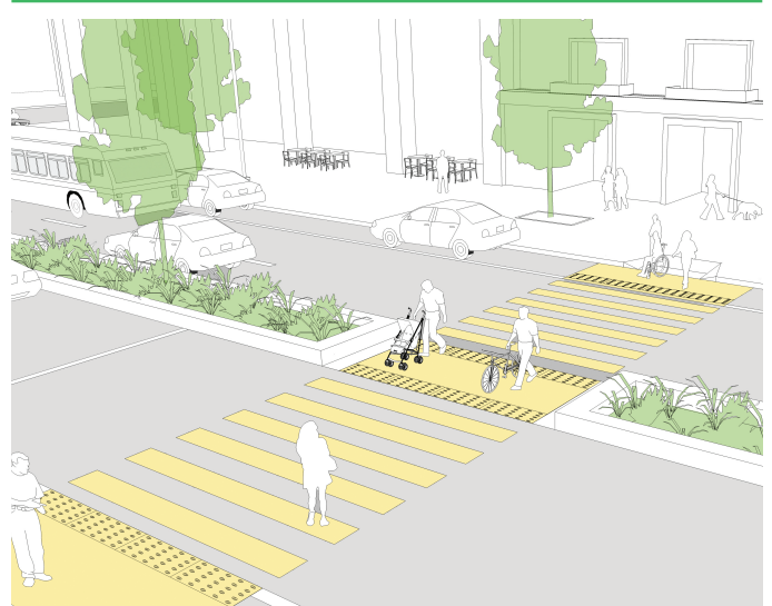
Raised center medians and pedestrian refuge islands can be used to reduce lane width for vehicles, even on relatively narrow streets. They can also be used to organize traffic at intersections or to block vehicle access.*
